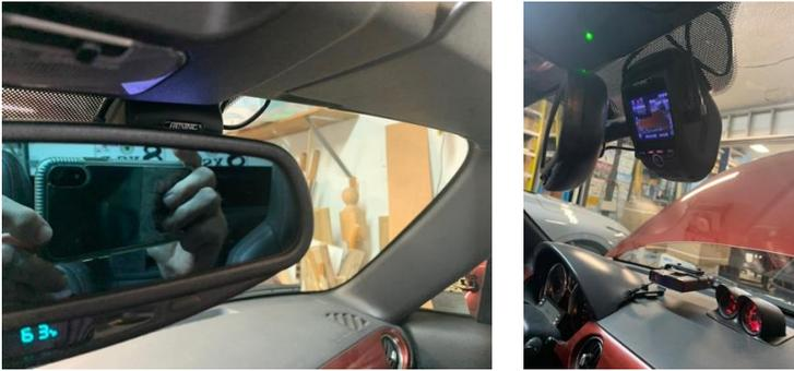
The camera is hard wired into the fuse box using “Add a Fuse”, fuse box adaptors. There are three circuits added in here for the camera, gauges and for the radar detector. The Add a Fuse gizmos make for a clean & safe installation. A switch was added to control the on/off function of the camera (the lit red ring). The camera can be left on for parking lot protection.
