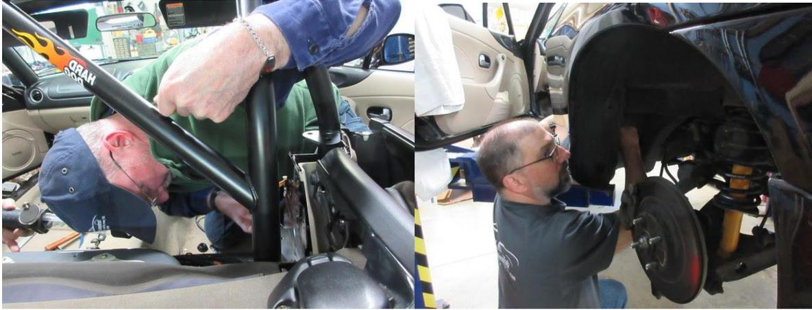
**Step 3**, finally, bolt the bar back in the car, spray some rust proofing on the exposed new nuts under the car and reconnect the wiring. Oh, don't forget to run the wires **BEFORE** bolting the bar in the car so that they'll have enough slack to be reconnected (don't ask how we know this).
