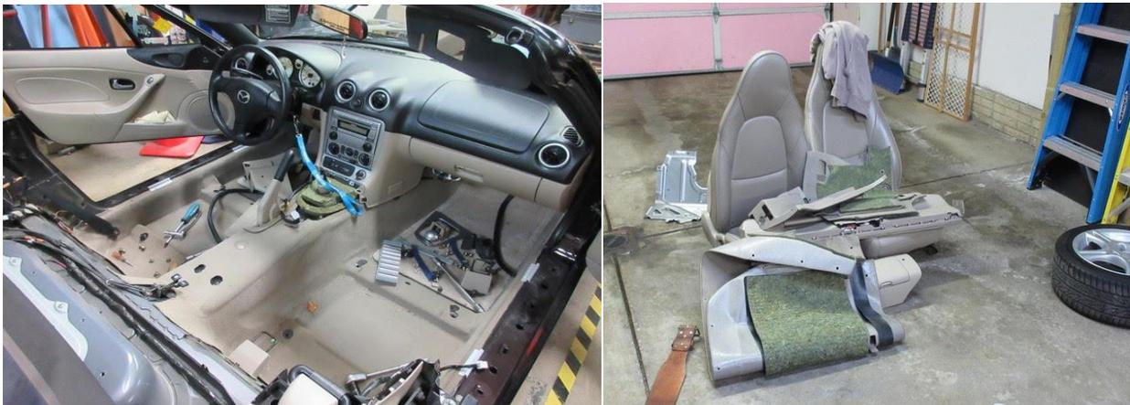
**Step 1**, remove the interior: note that on some Miatas the seat belt reel must be removed and wiring disconnected during this step as well. Make a big pile of parts and fasteners (in marked bags) behind the car. Remove both rear wheels and add them to the pile.
