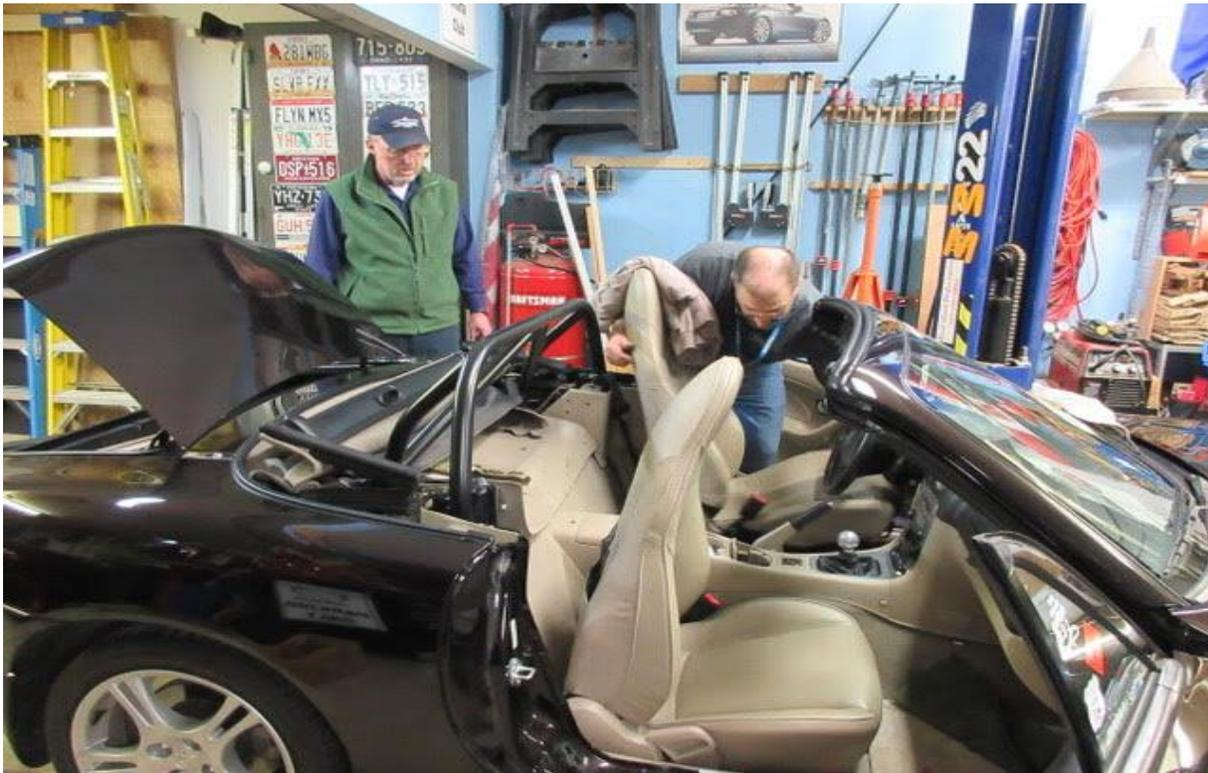
**Step 4**, Put the seats & console back in, trim the rear shelf carpet and plastic panels to fit around the new roll bar & install those.
