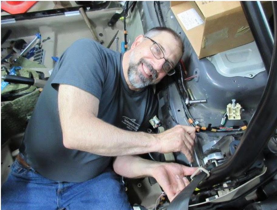
**Step 2**, put the bar in the car, carefully position it and mark all of the holes. Remove the bar (you'll get used to putting the bar in and taking it out and the extra hands make it much easier), pilot drill the holes & then drill to 3/8" diameter. Don't forget to be happy in your work & smile...or is that a grimace? No matter, just get it done.
