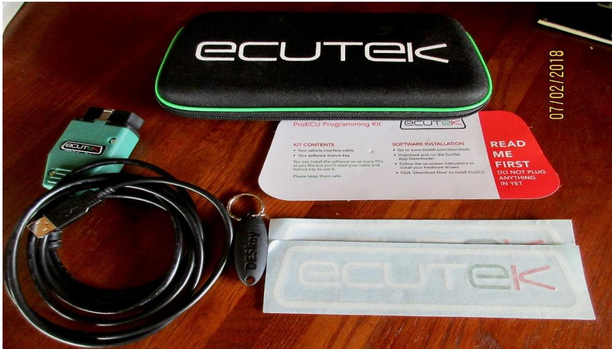
Here's the whole ECUTEK Programming Kit. Packed in the soft case is the ECU/computer interface cable (coiled on the left), the license dongle (thumb drive) a couple of stickers (you must have stickers) and the instruction sheet (read it!). Once you have this in hand you can get going on your tune.
