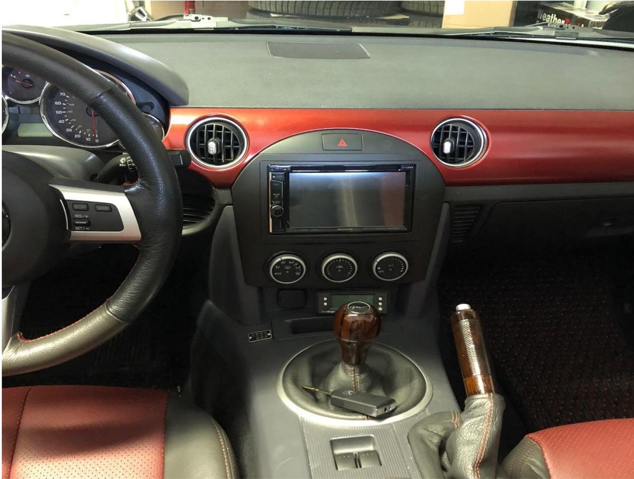
The new head unit & surround mounted in the dash...looks factory. The mic for the Bluetooth is behind the steering wheel.
