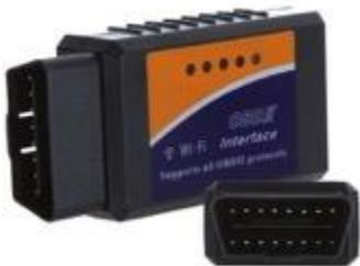
Above, plug in interface for the OBDII code reader.
